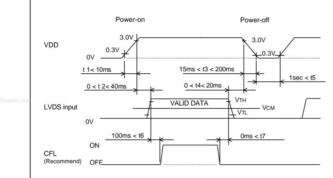
When the power is off, LVDS input must be kept at either low level or high impedance.
